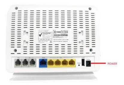
5. Use the yellow Ethernet cable (included with the modem) to connect the modem to the NCD. Use the blue WAN port on the back of the modem and connect this to the yellow GATEWAY port on the back of the NCD
