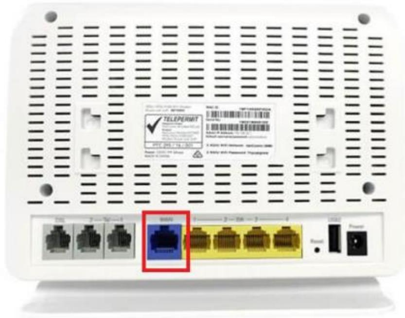
5. You can connect computers or other devices to the yellow LAN ports on the back of the device.
