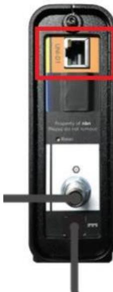
4. Locate the yellow Ethernet cable that was provided with your new modem and connect it from the next available (or active) Uni-D port to the blue WAN port on the back of your new Netcomm modem. Please see image below:
