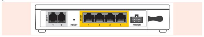
Using an Ethernet network cable, connect your router from its WAN port to the relevant Uni-D port on the NBN Connection Box. We generally activate the next available Uni-D port – starting with Uni-D 1. We will detail your Uni-D port number in our emails to you.
